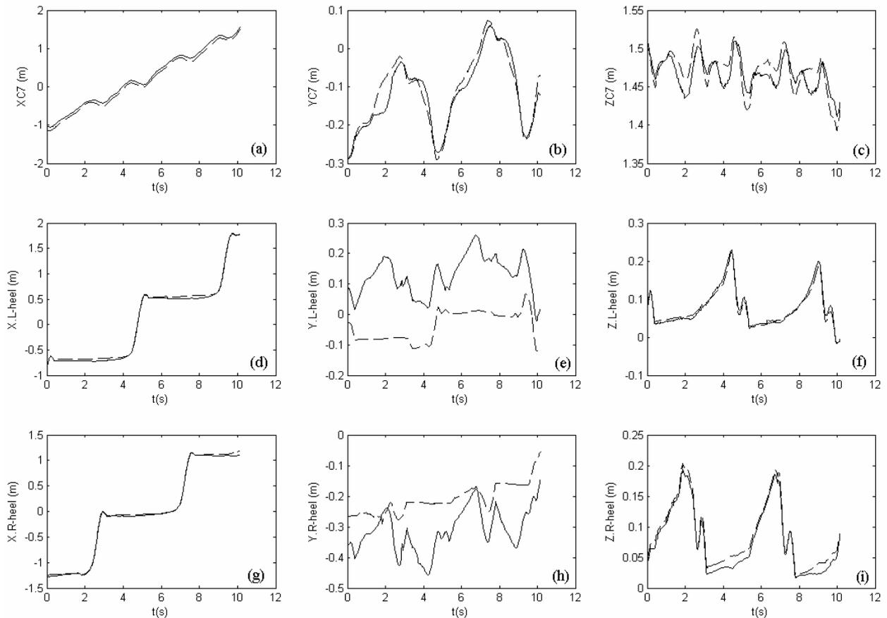
**Figure 4.** Comparison of the 3D trajectories of the end effectors predicted by the model (solid lines) and obtained from the experiment (dash lines) considering the lower trunk segment as the reference: C7 (top), L-heel (middle), R-heel (bottom)
