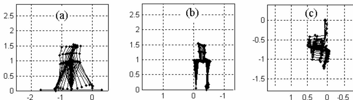
**Figure 5.** Stick figures of the 4 rigid body segments (trunk, pelvis, two legs) based on the 3D coordinate measurement during a representative swing phase: ( a) Sagittal plan, (b) Frontal plan, (c) Horizontal plan
