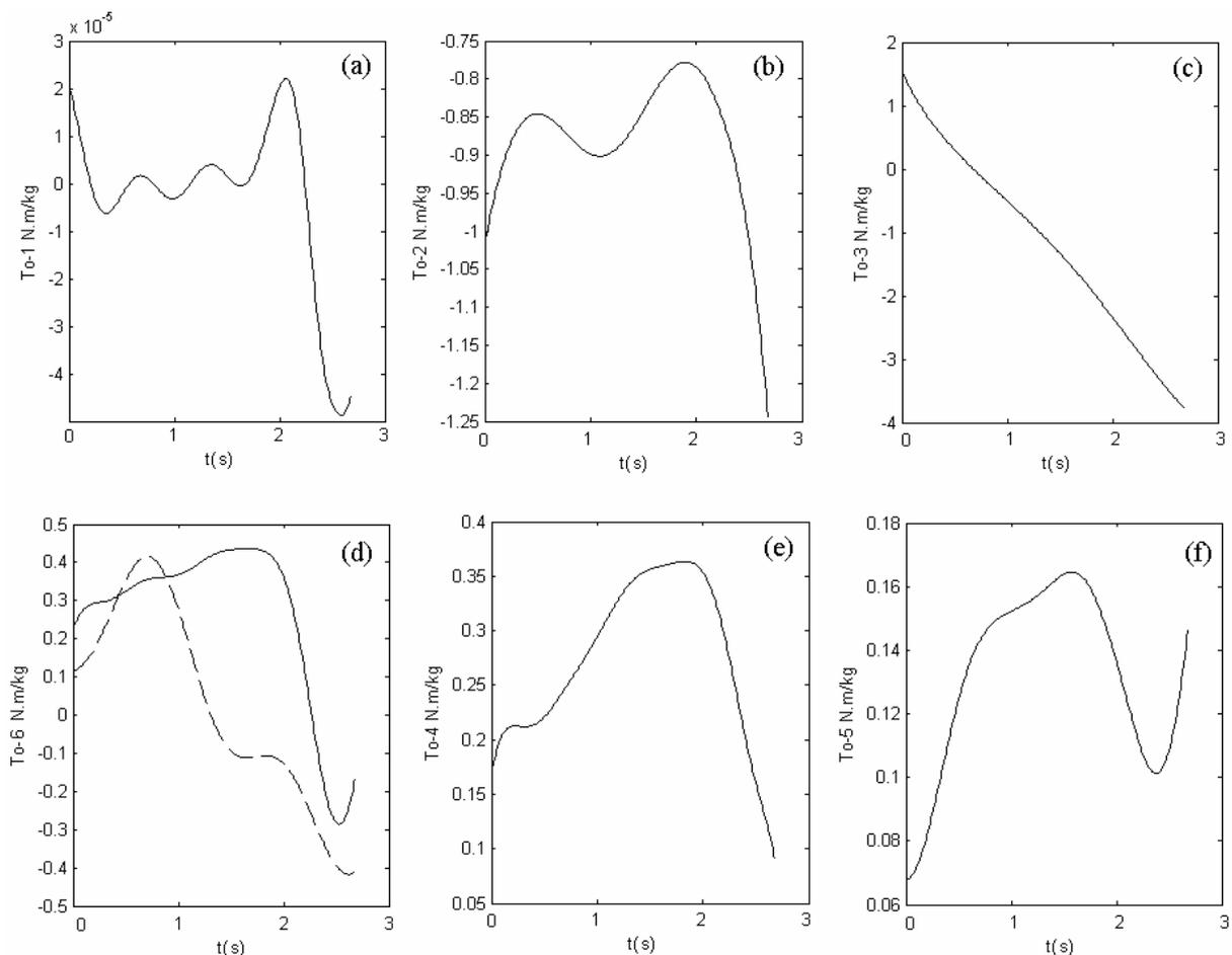
**Figure 6.** The torques related modeled paraplegic gait during a representative swing phase (solid lines) compared with the normal walking just in the hip joint (dash line). (a) whole body axial rotation around the stance leg,  $\tau_1$ , (b) whole body lateral tilting over the stance leg,  $\tau_2$ , (c) whole body forward inclination over the stance leg,  $\tau_3$ , (d) hip flexion of the swing leg,  $\tau_6$ , (e) trunk anterior bending,  $\tau_4$ , (f) trunk lateral bending,  $\tau_5$
