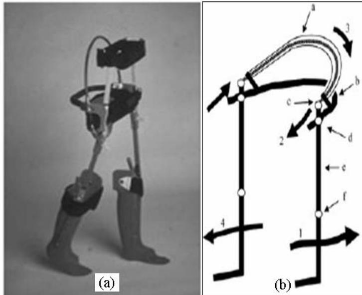
**Figure 1.** (a) Advanced Reciprocal Gait Orthosis. (b) Elucidation of the Reciprocal Cable functions in an ARGO structure.
