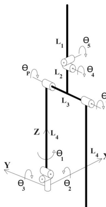
**Figure 3.** A four segment model, including trunk (L1), pelvis (L2 & L3), and left and right legs (L4) was used to describe the paraplegic ambulation.
