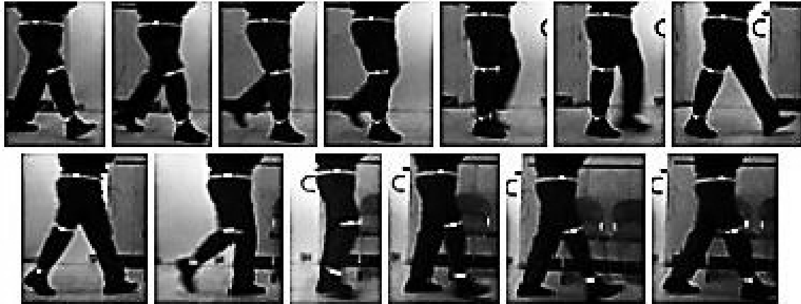
Figure 1. Gait analysis of a full gait cycle with three reflective markers (post-TKR subject)
