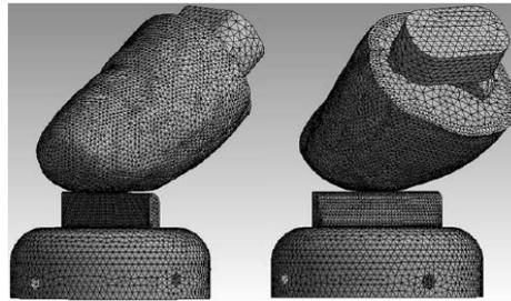
Fig 6. Networking of snap-fit and thumb model
