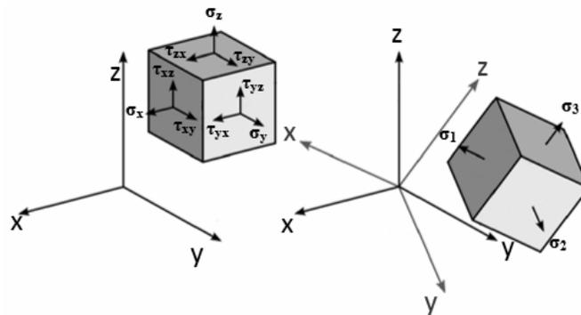
Fig 7. normal, shear, and primary stresses
