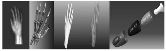
Fig 2. Steps of three-dimensional modelling of finger from CT scan to Segmentation and creating the model with CATIA
