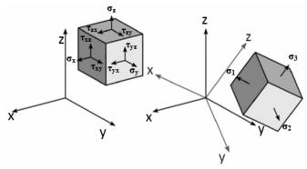
Fig 7. normal, shear, and primary stresses
