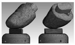
Fig 6. Networking of snap-fit and thumb model
