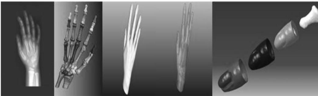
**Fig 2.** Steps of three-dimensional modelling of finger from CT scan to Segmentation and creating the model with CATIA
