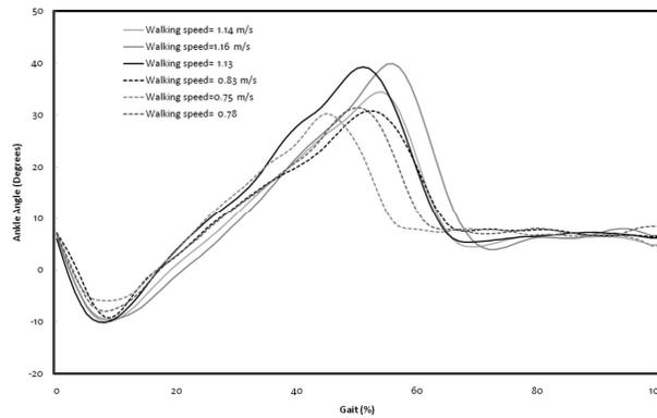
**Fig 4.** The prosthetic side ankle angle versus gait cycle percent for six walking trials with slow (dashed lines) and normal (solid lines) speeds
