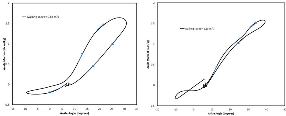
**Fig 3.** The prosthetic side ankle angle versus moment at slow (0.83 m/s) and normal (1.3 m/s) speeds.
