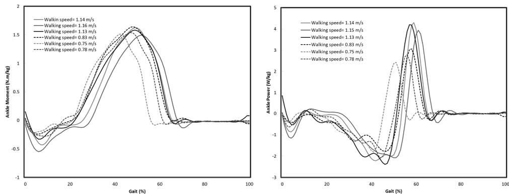
**Fig 5.** The prosthetic-side ankle moment (left) and power (right) versus gait cycle percent for six walking trials with slow (dashed lines) and normal (solid lines) speeds
