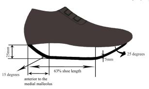
Fig 1. Structure of rocker shoe
