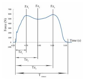
• Fz<sub>1</sub>: first maximal vertical force, Fz<sub>2</sub>: minimal vertical force, Fz<sub>3</sub>: second maximal vertical force, Tz<sub>1</sub>: time to Fz<sub>1</sub>, Tz<sub>2</sub>: time to Fz<sub>2</sub>, Tz<sub>3</sub>: time to Fz<sub>3</sub> and Tstance: stance time.
