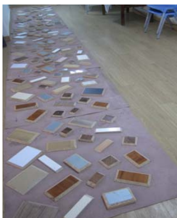
Fig 2. The irregular walkway created by Wooden Pieces which were randomly oriented beneath a dark carpet surface
